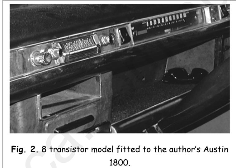
**Fig. 2.** 8 transistor model fitted to the author's Austin 1800.
