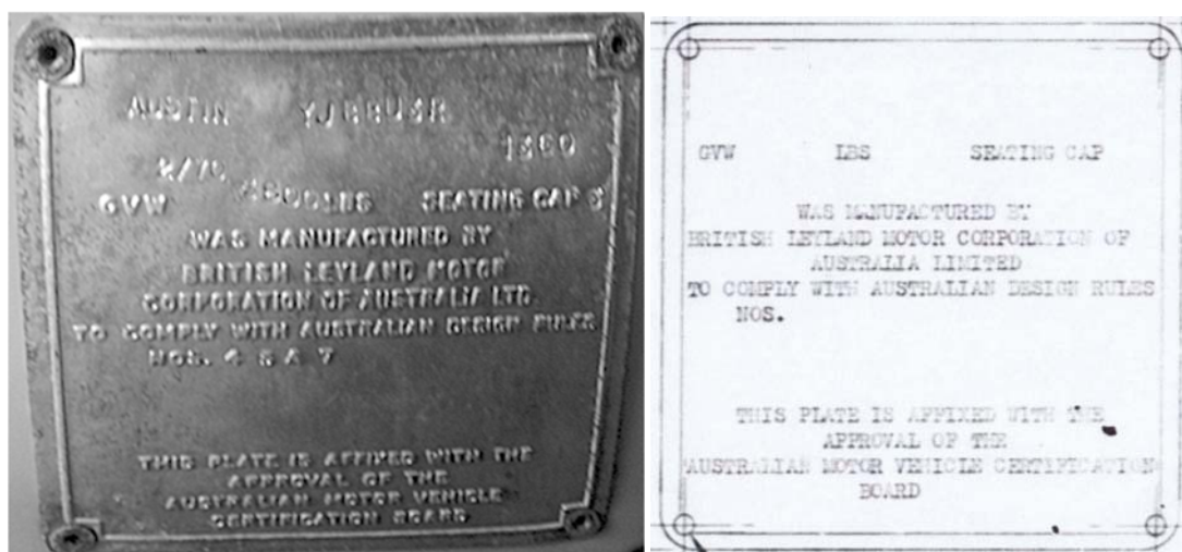
Fig. 4.1.2.1 Compliance Plate Type 1 introduced in 1970.
